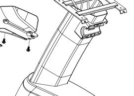
Attach the back console cover (40) to the console using the bolts.
