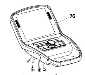
Attach the console (76) onto the front post using the cross bolts (39).
