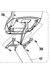
Attach the console (76) onto front post (17) using the fixing bolts (39).
