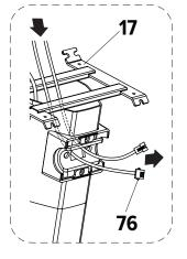
Thread the console cable into the front post (17) and then out of the handlebar mount hole like shown.
