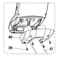
Attach the back console cover (40) to the console using the fixing bolts (39).
